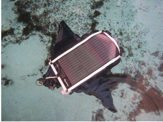
Figure 10. Underwater Testing of Solar Ray with Right Wing Flapping (Note ripple).
