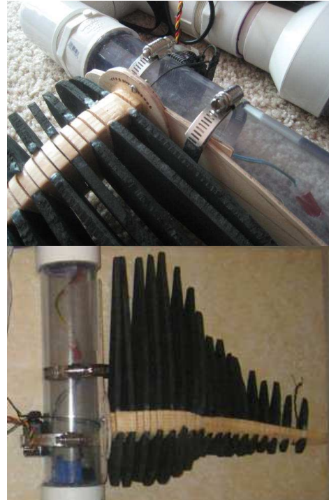
Figure 5. Wing Internal Frame with Angle of Attack Adjustment and Servo Actuated Pull-Pull Mechanism.
