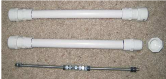
Figure 4. System for Buoyancy Fine Tuning and Center of Gravity Adjustment.
